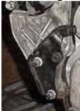
This is the mount bracket that attaches to the alternator bracket.
