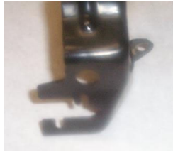
Cable slots are too large for the 95's
